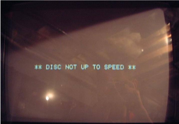
This does NOT mean that your player is bad! (Although it could mean that). Be sure that you "Y" cable is connected correctly. Also, if you can verify your player is working (see the NTSC section for plugging the image directly into the monitor), then you may have an issue on the GSI board.
